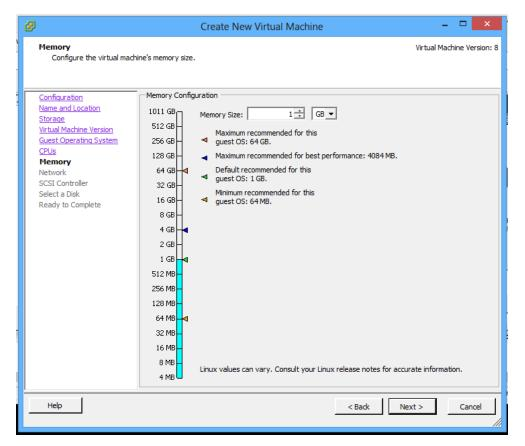
The next two screens (Figure 2.41 and Figure 2.42) allow you to specify the initial amount of RAM and processor resource to assign to your virtual print appliance.
