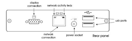
Connect the box to your network by plugging an ethernet cable into the network port on the back of the unit (Figure 2.2).
