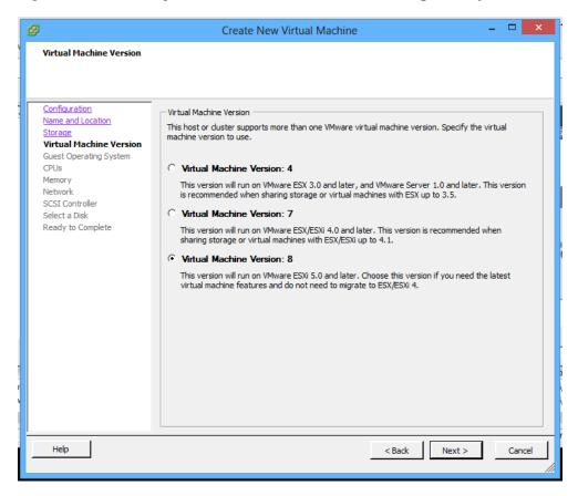
The Virtual Machine Version window allows you to specify the hardware compatibility for the virtual machine. This may be a consideration if you wish to move your virtual machine to older versions of VMware ESXi or to other VMware infrastructure products. In our example, we leave it at its default of **8**.
