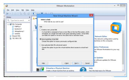
In the next window (Figure 2.27) you have the option to **Create a new virtual disk**. This would create an *empty* disk, which would then need to have the operating system installed (perhaps from a dvd or cdrom). Because you are using a pre-populated disk file supplied by WML, you should click on **Use an existing virtual disk**, which will open the next window, shown in Figure 2.28.
