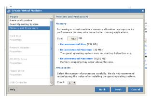
This screen (Figure 2.6) allows you to specify the initial amount of RAM and processor resource to assign to your virtual print appliance. Specify a minimum of 256 MB of RAM. Some applications may require more memory to run correctly, but 256 MB is sufficient for simpler tasks and short documents.
