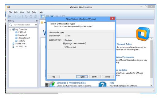
Figure 2.26. Selecting the virtual I/O controller type.
