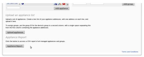
Towards the bottom of the Appliances and Groups page, there are two additional sections, shown in Figure 11.2. **Upload an appliance list** provides an interface to use a text file to populate the **Network appliances** list. **Appliance Report** generates a full report of the system and is covered later in this section.
