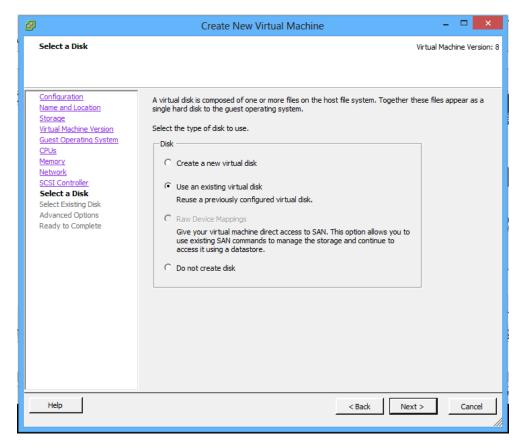
In the next window (Figure 2.45) you have the option to **Create a new virtual disk**. This would create an *empty* disk, which would then need to have the operating system installed (perhaps from a dvd or cdrom). Because you are using a pre-populated disk file supplied by WML, you should click on **Use an existing virtual disk**, which will open the next window, shown in Figure 2.46.
