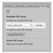
Select the form from the menu highlighted in Figure 6.33. Press the **Activate** button. The form should appear on the canvas, as shown in Figure 6.34.
