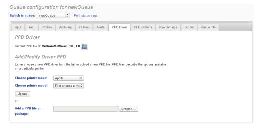
Figure 5.23: The most important configuration setting for the queue is the PPD driver. This is where you define how the PdfPlus should format the document before it is sent to its destination. The PPD driver selects which of the PdfPlus's internal printer driver filters is used to convert the job from the PdfPlus's internal format (PDF) into printer-ready output.
