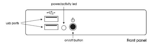
Plug the power supply into the back of the unit. Turn the PdfPlus on using the button on the front of the unit (Figure 2.3). You should see the blue indicator light come on.
