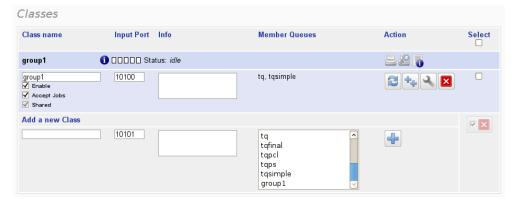
To add a class, enter a name for the class, and select at least one member for the class. Multiple queues may be selected by holding down the control key. The input port defaults to the next available port number, starting at 10100. Click on the add button ( ) to add the class to the system.
