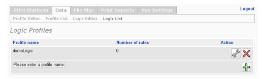
Add a new profile by filling in the logic profile name, and pressing the add button (). The new profile will appear in the list, as shown in Figure 8.2. Click on the configure button () to access the logic editor page for the new logic profile. The empty logic profile is shown in Figure 8.3.
