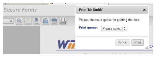
When the form is complete, press the print button (). A dialog will open allowing you to select the destination printer (this is a list of all the queues which are configured on the DataGateway). Click **Print** and the form will print to the selected printer.
