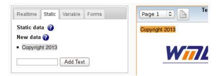
Figure 7.13 shows the static data tab, with a single static data element containing the text "Copyright 2013". To place the element, drag and drop it in the usual way. Multiple copies of the static element may be placed on the canvas.
