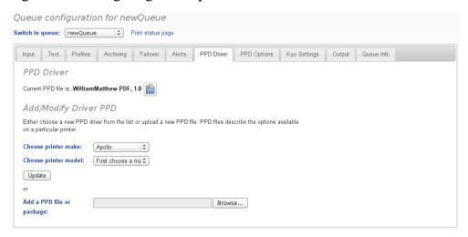
Figure 6.25: The most important configuration setting for the queue is the PPD driver. This is where you define how the DataGateway should format the document before it is sent to
