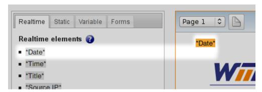
Dates and times are *realtime* data text elements. Select the **Realtime** tab. Drag a date element onto the canvas and position it as shown in Figure 7.35. Do the same for a time text element.
