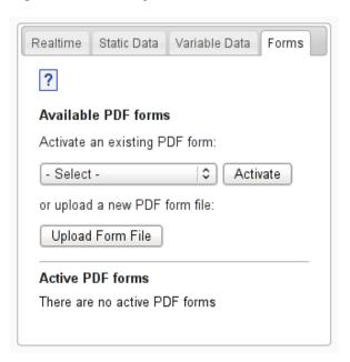
Any PDF forms which you wish to use with the DataGateway must first be uploaded to the appliance. Click on "Upload Form File" and browse to your PDF. The file will be uploaded to the DataGateway and processed by the internal software to ensure it can be successfully parsed.
