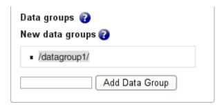
Figure 7.19 shows the result of entering "datagroup1" into the data group text field and pressing "Add Data Group". A heading "New data groups" has appeared with a single item "/datagroup1/". Note the slash characters enclosing the data group name. These indicate that this is a data group element and are not part of the data group name.
